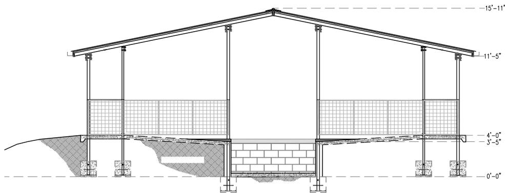
Figure 7: Commercial dry-litter piggery schematic Source: (American Samoa, EPA)
