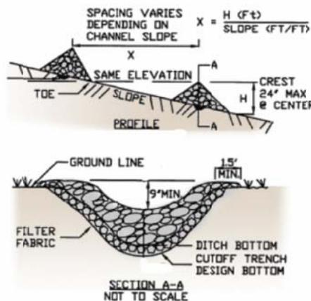
Figure 8: Stone check used in Compact Road, Palau
