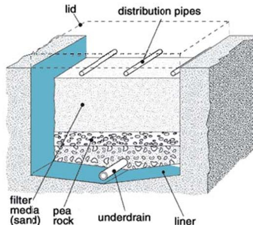
Figure 5: Sand filter for septic tank system. Source: (University of Minnesota)
