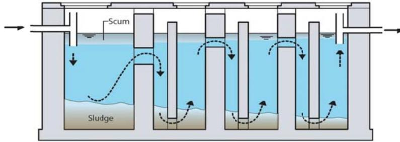
Figure 4: Anaerobic Baffle Reactor. Source (Morrell & Diener, 2006)
