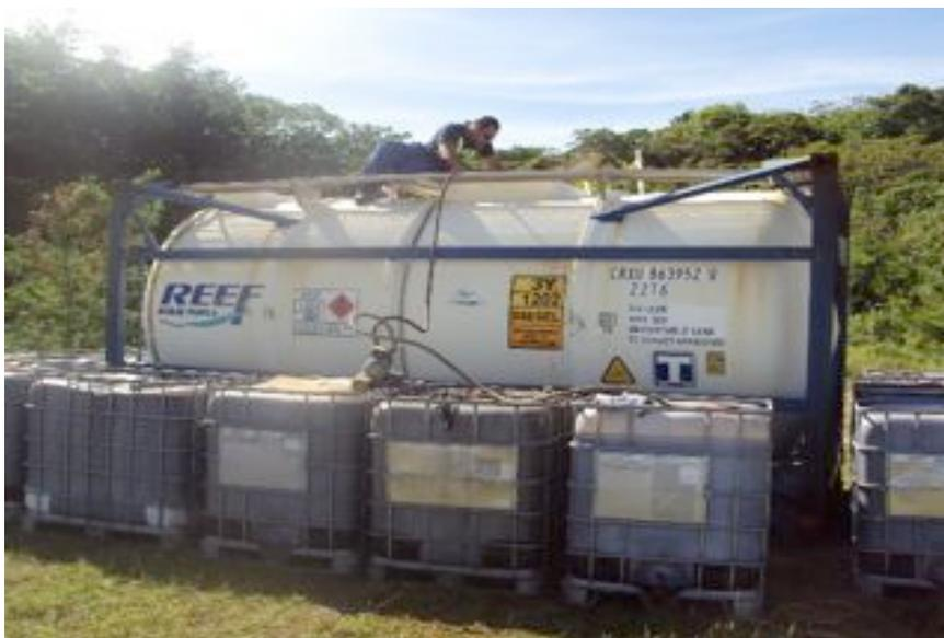
**Figure 8:** Waste Oil transfer for transport
